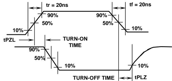
FIGURE 1. WAVEFORM CHANNEL BEING TURNED ON, OFF
